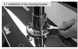
Place four spring rings on the threaded bolts, and tighten each with a cap nut using wrench.
