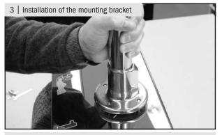
Person 1 turns the mounting bracket in such a way that the two headless screws of the base flange of the mounting bracket points to the rear side of the machine. Person 1 positions the mounting bracket on the four threaded bolts correctly. When placing make sure that the power cable of the mounting bracket is not jammed.
